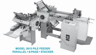
The Baum 2015 is the perfect transition from tabletop to floor-model folding. You can fold the same jobs as your tabletop, but with higher production capacity. The 2015 easily handles 8-1/2" x 11" to 14" x 20" nominal sheet sizes.
